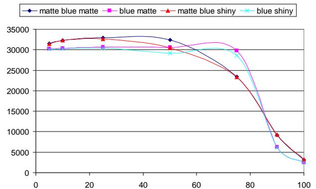
Fig. 9: Scanning results for blue samples (RAL 5017)
