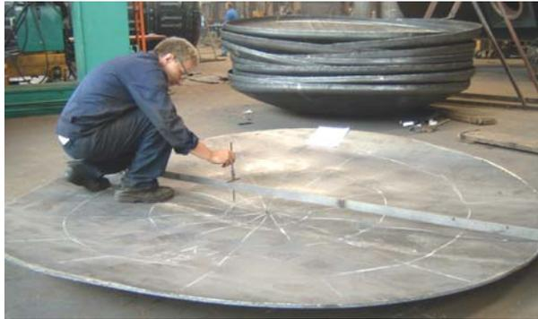
Figure 4. Measurement of buckled plate geometry.
