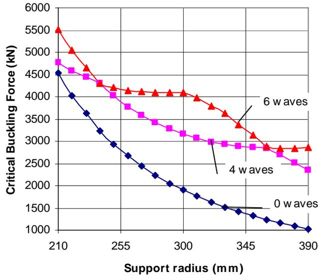
Figure 3. Critical buckling force for different support radius.
