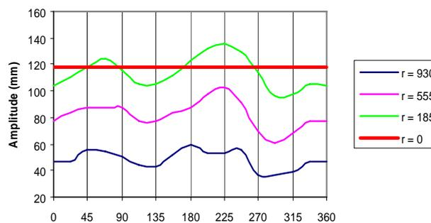
Figure 5. Example of buckling mode shape with 4 wrinkles
