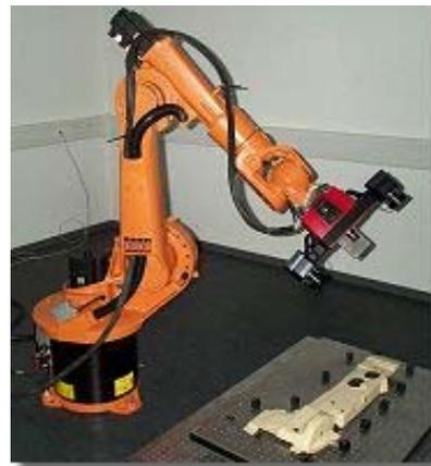
Fig.2. 3D Laser Scanner (www.gom.com)
