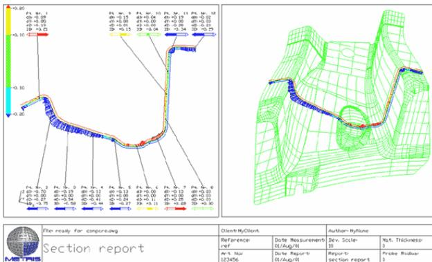
Fig. 5. Tolerance checking (www.metris.com)
