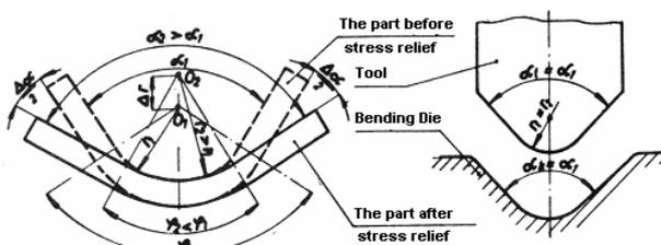
Fig.1. Elastic springback [1]
