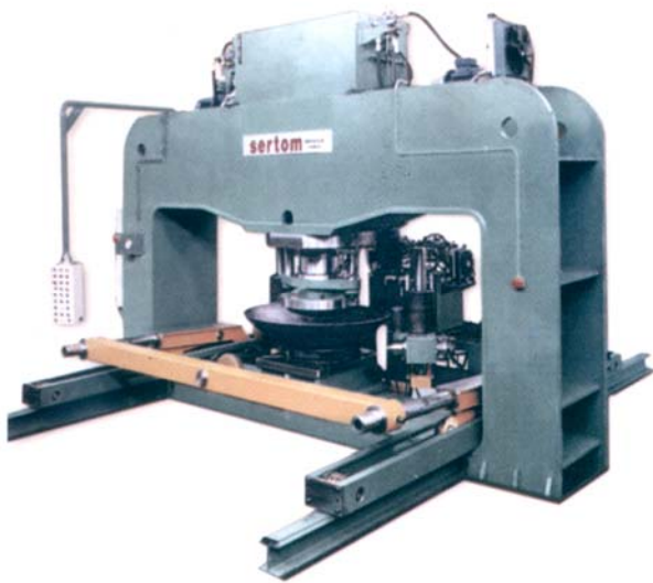
Fig. 1. Incremental forming press P2MF 200x4 - Sertom.
