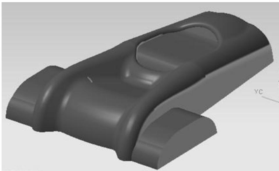
Figure 11: CAD model for upper part of redesigned sling.
