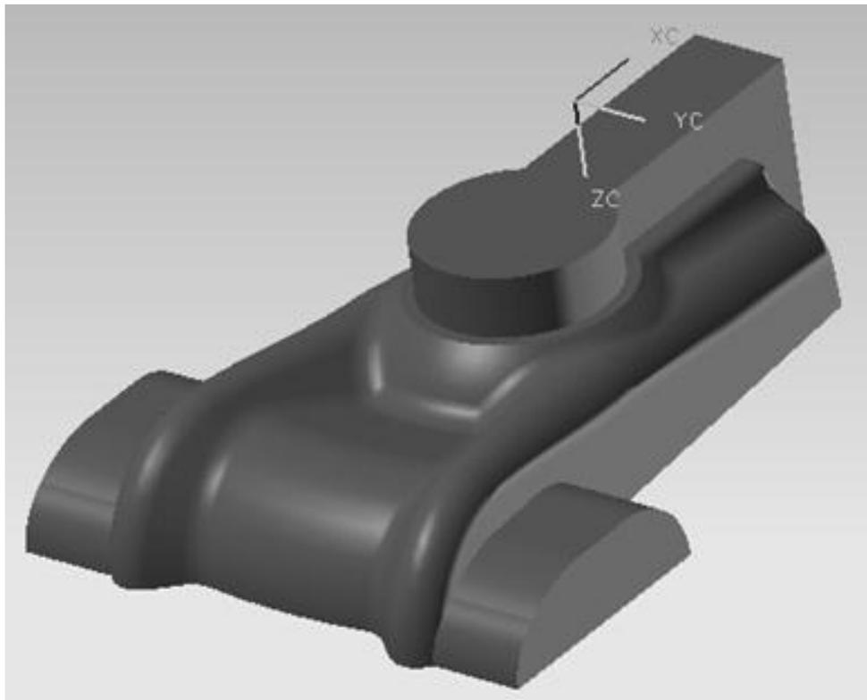
Figure 10: CAD model for lower part of redesigned sling.
