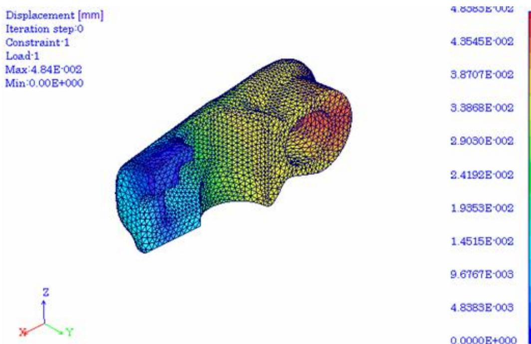
Figure 9: Deformation of sling under tension.
