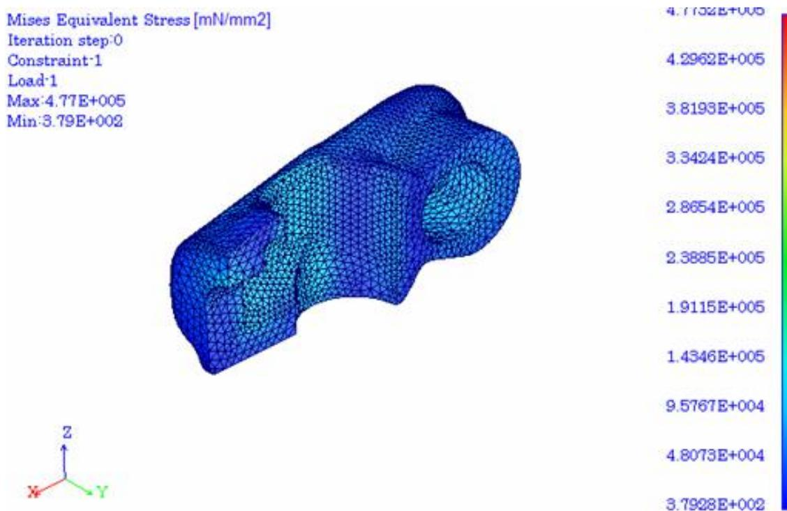
Figure 8: Equivalent stress distribution in redesigned sling.
