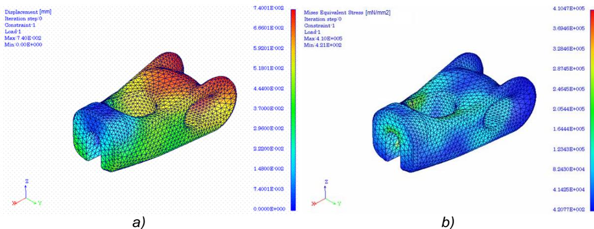
Figure 3: Initial static analysis results: a) displacements, b) equivalent stress.
