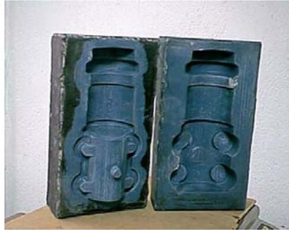
**Figure 3:** The casting model's negative – 2 halves
