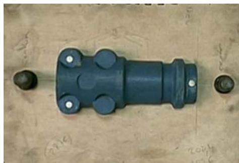
**Figure 5:** The model on pattern plate
