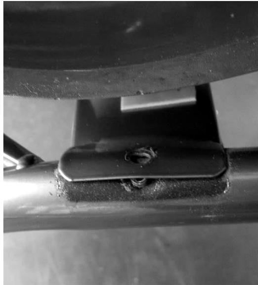
Fig. 5. Failed riveted joint
