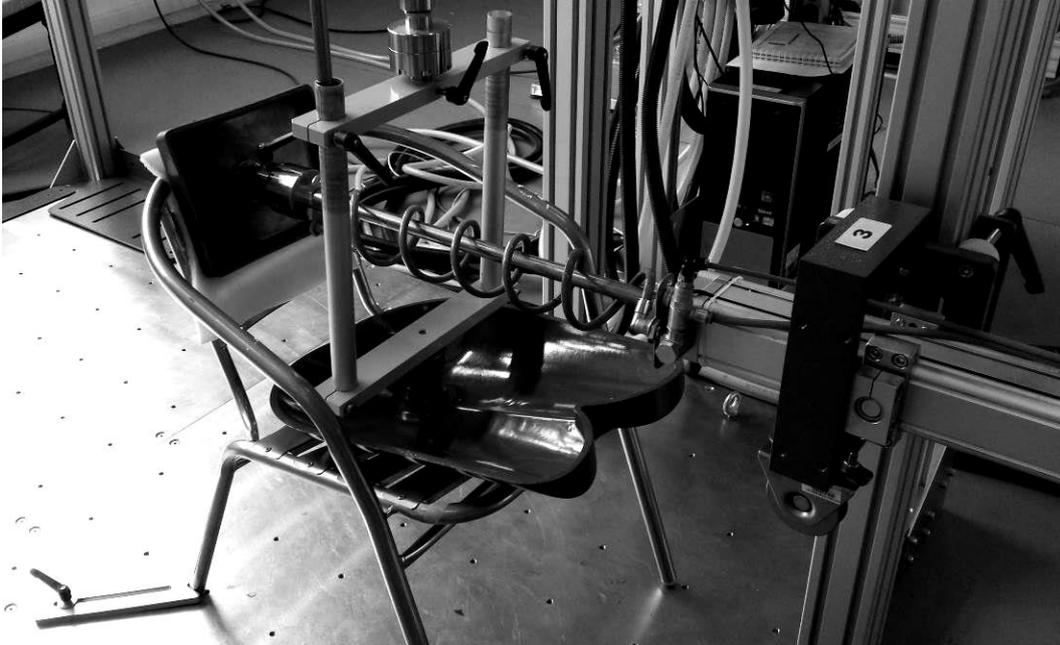
Fig. 2. Testing chair durability
