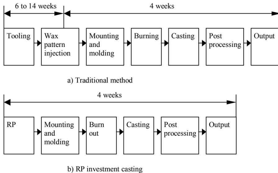
Figure 1. Comparison between traditional methods and RP in investment casting process
