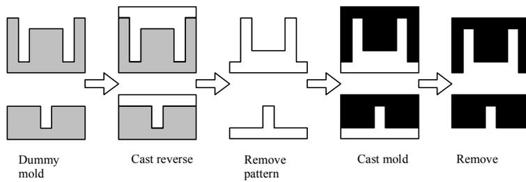
Figure 4. Double reverse tooling method
