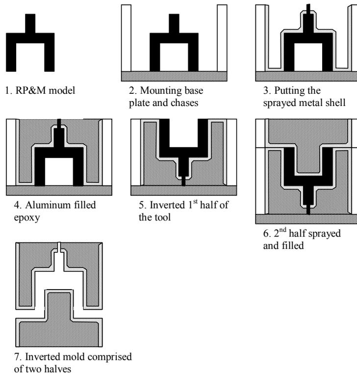
Figure 3. Spray metal molding process for tove production
