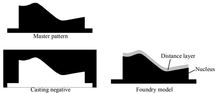
Figure 8. Plastic Resin casting scheme
