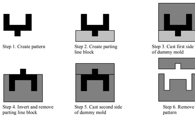
a) Single reverse to create dummy molds
