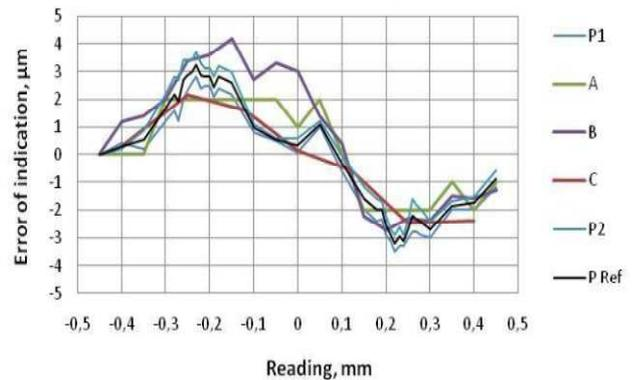
Fig 4: Dial gauge, comparison of error of indication (upward) for each participant, A, B and C.
