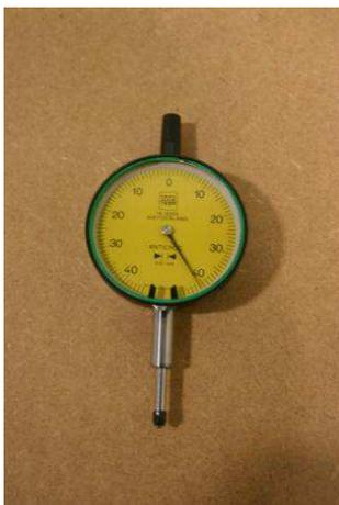
Fig 1: Dial gauge, analogue: TESA, Switzerland
