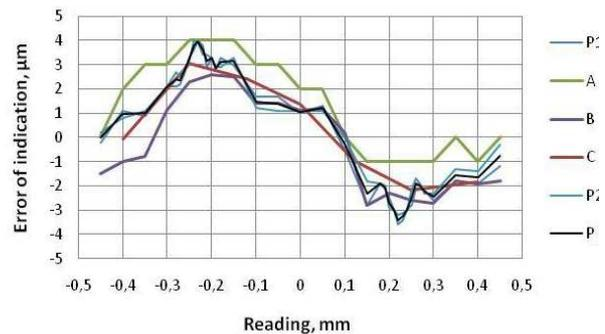
Fig 5: Dial gauge, comparison of error of indication (downward) for participated laboratory, A, B and C.
