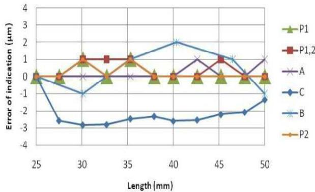
Fig 3: External micrometer, comparison of measurement of error of indication for each participant, A, B and C.
