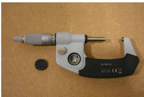
Fig 2: External Micrometer, digital: Mitutoyo, Japan
